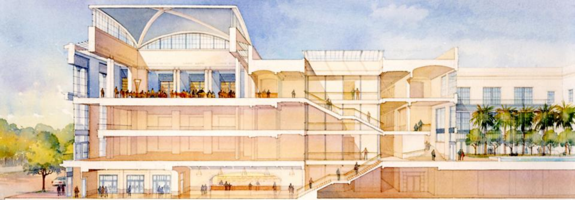
3-Dimensional Section through Grand Reading Room and Courtyard – Competition Entry
