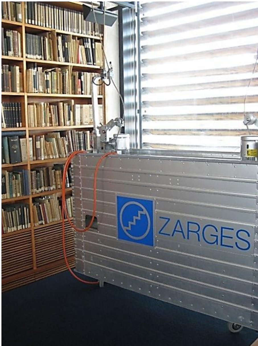
The fixed slats require special window cleaning equipment
